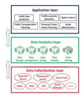
Data collection layer: The data collection layer is the design's premise as it gives the upper layer the vital data. The data originate from a variety of sources such as loop locators, microwave radars, video observation, remote sensing, radio frequency identification data, and GPS, etc. Insights on Big Data collection will be presented in the following areas.
