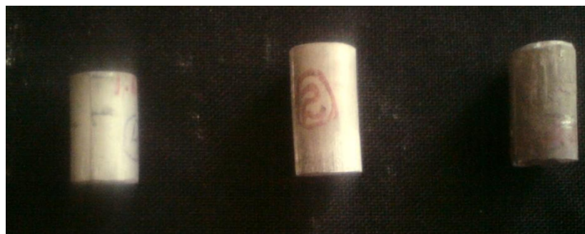
Figure 4. Pins Compacted at 390 MPa
