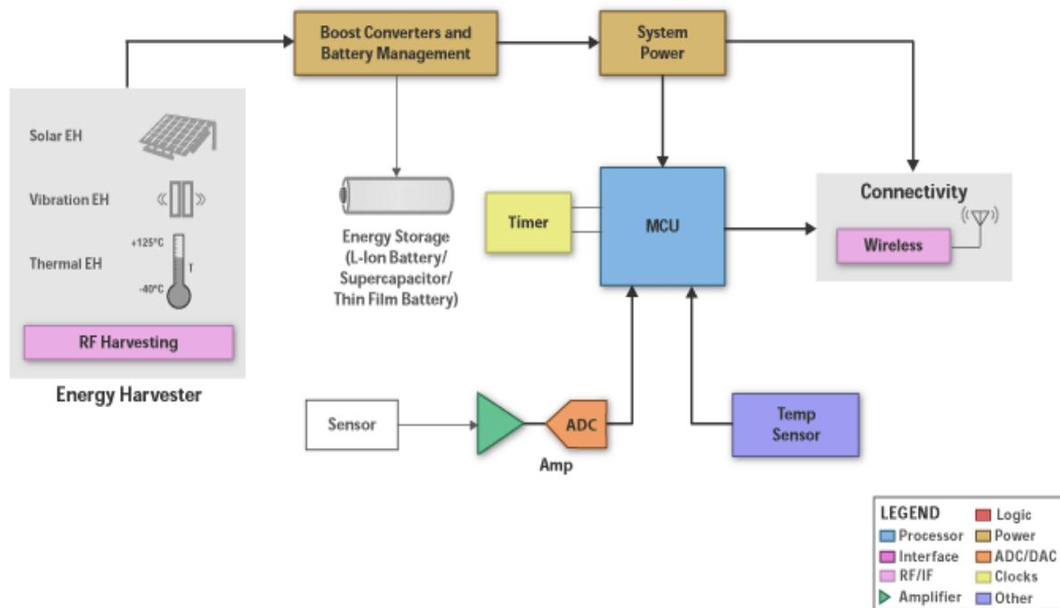
Fig.2: Energy Harvesting Block Diagram.
