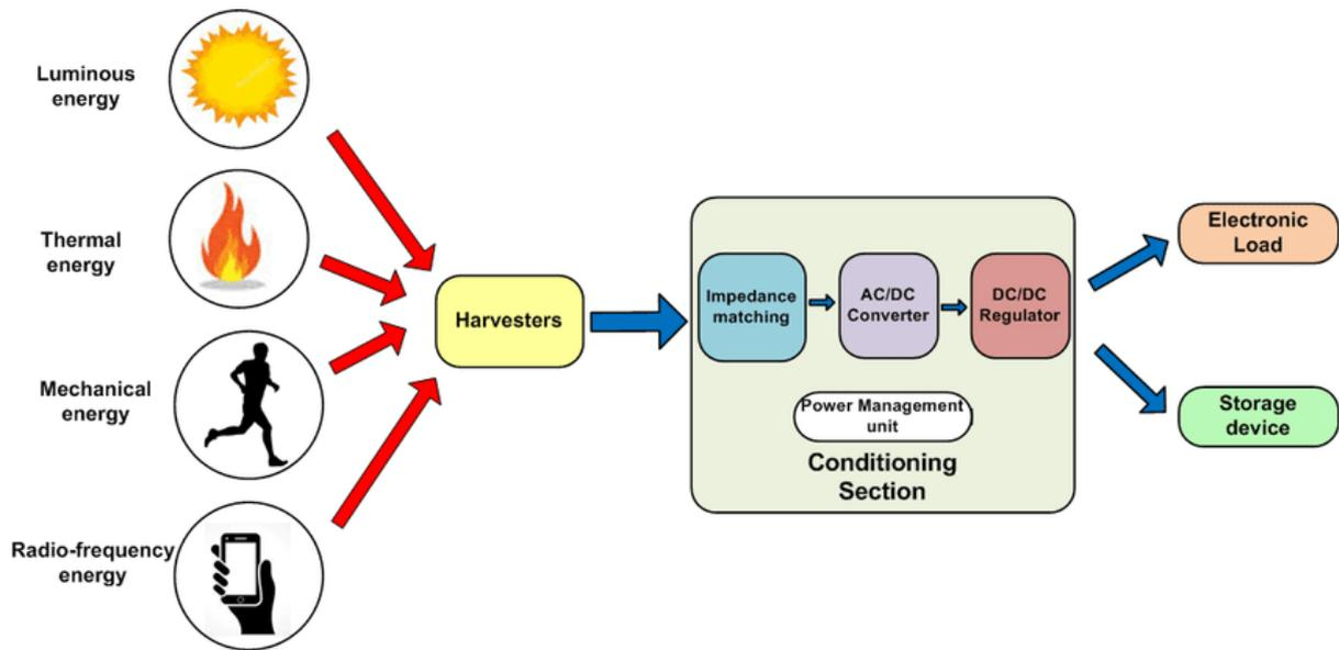
Fig.4: Block diagram of a generic energy harvesting system Diagram
