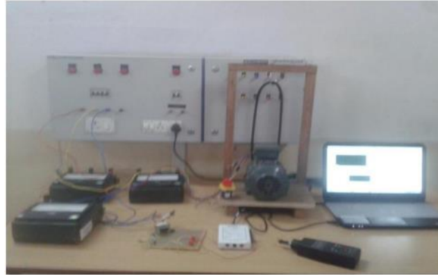
Figure 1: Configuration for Identifying Stator Winding Short Circuit Faults
