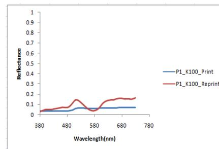
Fig11: Reflectance Spectrum of Solid Black for Printer1 (P1)
