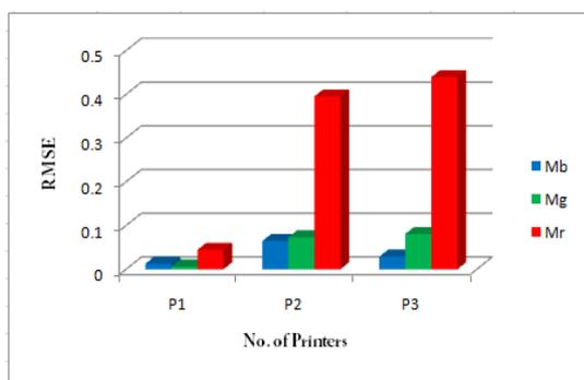
Fig19: RMSE values of Solid Magenta (between reference and test samples) for the three Printers
