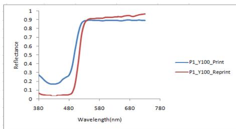
Fig8: Reflectance Spectrum of Solid Yellow for Printer1 (P1)
