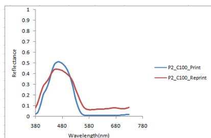
Fig3: Reflectance Spectrum of Solid Cyan for Printer2 (P2)
