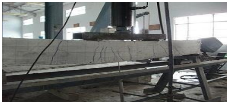
Figure 4. Beam test setup under cyclic loading
