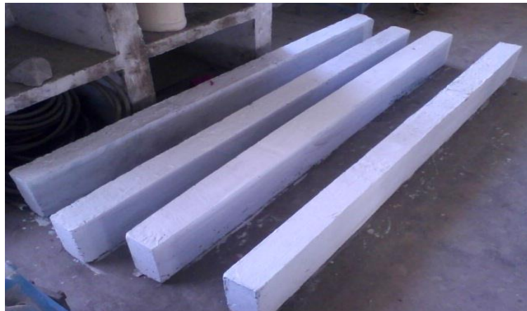
Figure 2. Beams Cured and whitewashed
