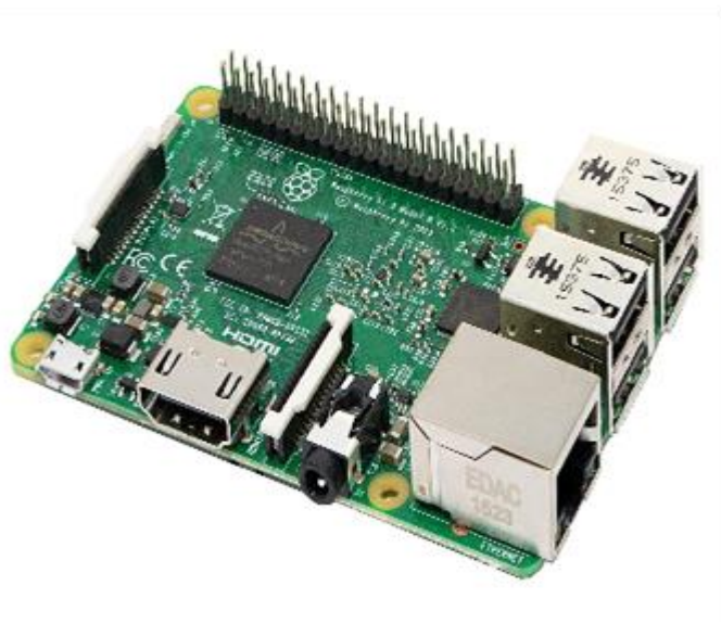
Figure 2 Raspberry Pi 3 model B
