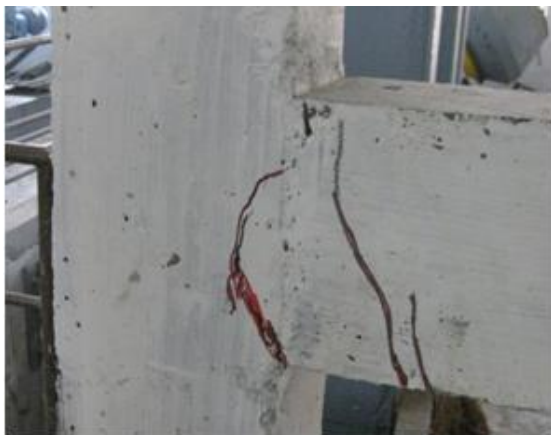
Figure.10 Failure Pattern of (PP3/4+Steel1/4)2.0 BC Joint
