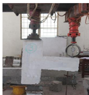
Figure.5 Beam Column Joint - Forward Loading
