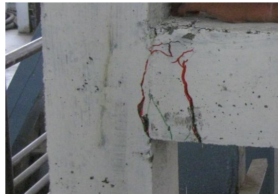
Figure.9 Failure Pattern of (PP1/2+Steel1/2)2.0 BC Joint
