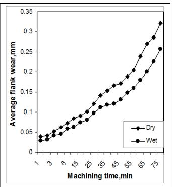
Figure 3(b) Growth of average flank wear in mm observed while turning E0300 steel by RCMT-10 T3-MO-4025 insert under dry and wet environments respectively.
