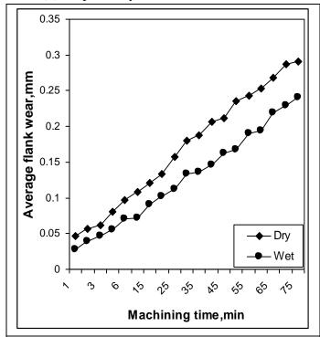
Figs. 3 (a) Growth of average flank wear in mm observed while turning E0300 alloy steel by RCMT-10 T3-MO-4025insert under dry and wet environments respectively.
