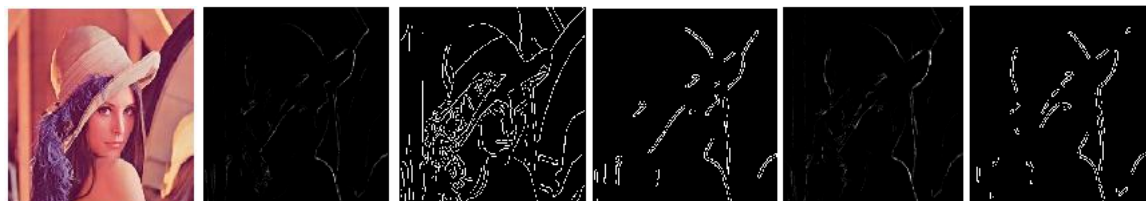
Figure4: (a) original image (b) ACO when ER=0.01 , (c) Canny (d) ACO with Canny (e) ACO when ER=0.5 (f) ACO with Canny.
