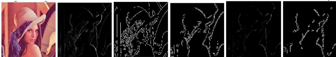
Figure5: (a) original image (b)ACO when PHY = 10^{-10} , (c) Canny (d) ACO with Canny (e) ACO when PHY = 1 (f) ACO with Canny.
