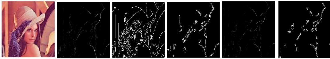
Figure3: (a) original image (b) ACO when \beta=0.03 , (c) Canny (d) ACO with Canny (e) ACO when \beta=2 (f) ACO with Canny.
